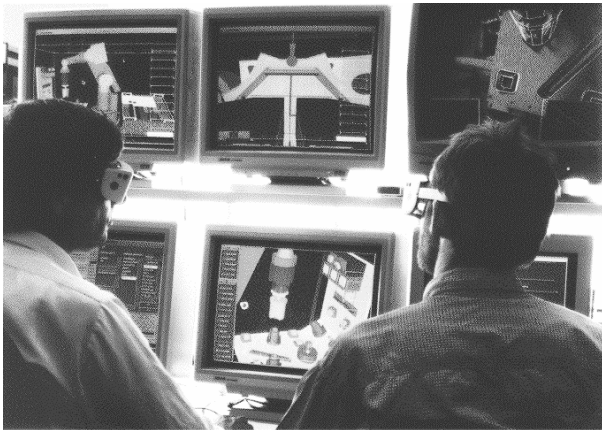
Figure 3 GUI of the universal programming and control station (MARCO)
