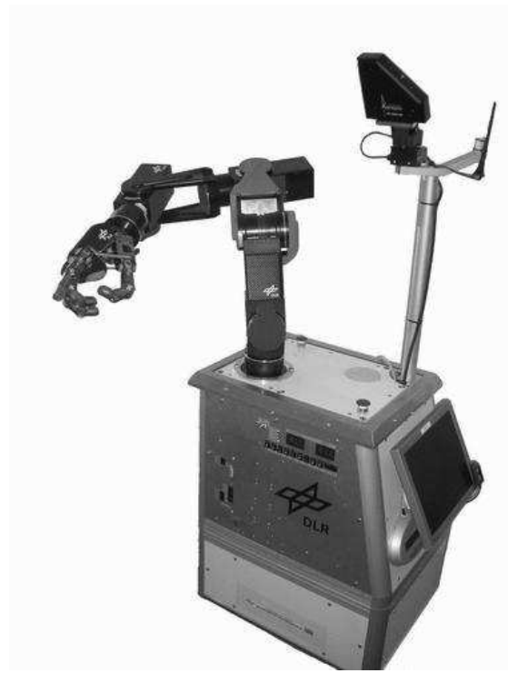
Fig. 1. The Robutler: a mobile hand-arm system with stereo cameras and laser scanner. The arm shown is the second generation of DLR's Light-Weight Robots.
