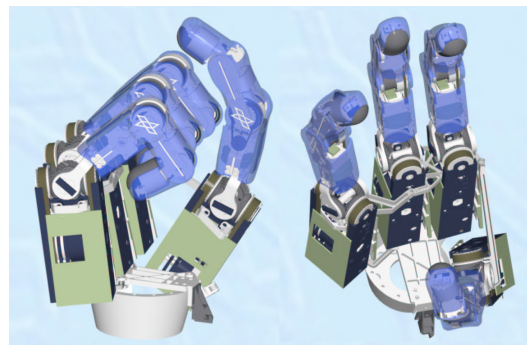
Fig. 7. Power (left) and precision (right) grasp configuration of the DLR Four-Finger Hand.
