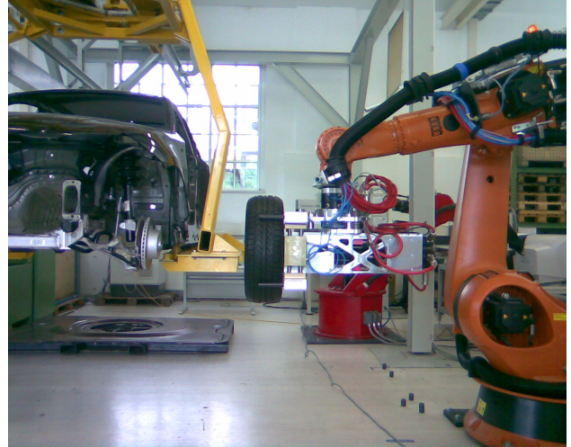
Figure 3: Experimental set-up at iwB for wheel assembly using a KUKA robot without linear axis .
