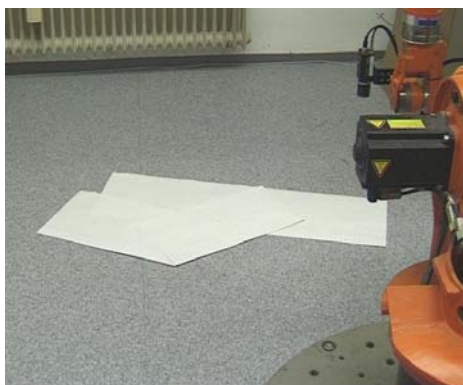
Figure 1. Originally the robot is programmed to execute a linear motion, back and forth. But image data of the robot-mounted camera are used to modify the desired path in order to track the edges of randomly spread sheets.
