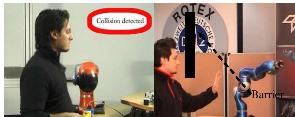
Fig. 11. Real collisions with the chest and arm were conducted up to a robot velocity of 2.7 m/s.
