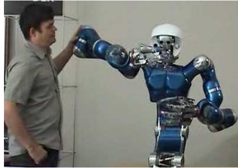
Fig. 14. Physical interaction with the DLR humanoid Justin
