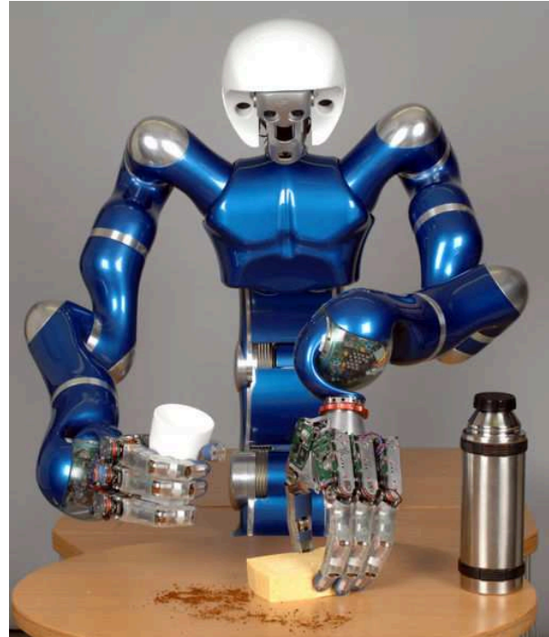
Fig. 1: DLR's Justin - a humanoid upper body using the lightweight robot technology.
