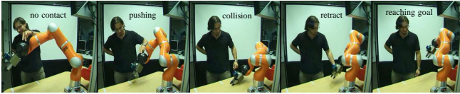
Fig. 4. Automatic recovery from physical collisions with real-time motion planning.
