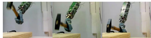
Fig. 15. Sequence of the DLR Hand Arm System driving a nail into solid wood using a 500 g standard hammer.
