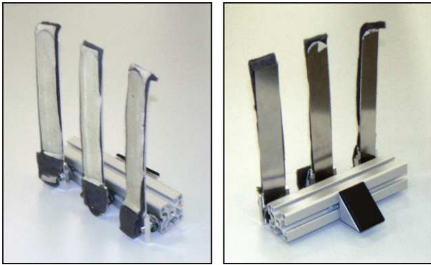
Fig. 3. Elastic dribbling hand used for the experiments with the DLR Lightweight-Robot III.
