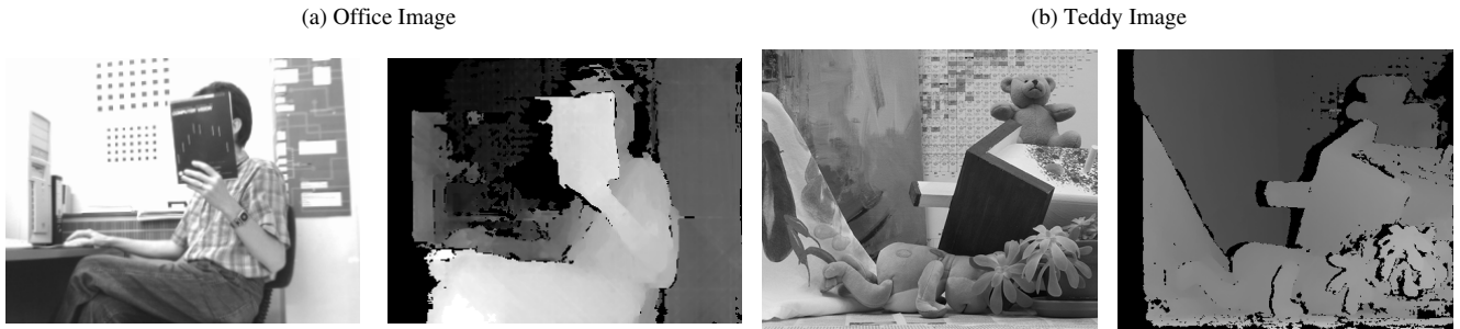
Figure 2. SGM results on images with untextured background areas. Black represents filtered ( i.e. invalid) disparities.
