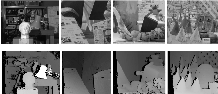
Fig. 2. Results of computing SGM on the GPU with mutual information and 5 hierarchical levels
