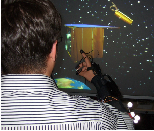
Figure 5: A human operator is evaluating the two tactile devices by exploring a virtual model of the German Micro-Satellite BIRD. The pose of the human arm and fingers are tracked optically by A.R.T. infrared cameras and visualized in the virtual world (yellow cylinder and hand at the top right corner).
