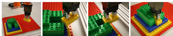
Figure 3: On-Site Setup task: Set parameters for fitting Lego brick in a notch.
