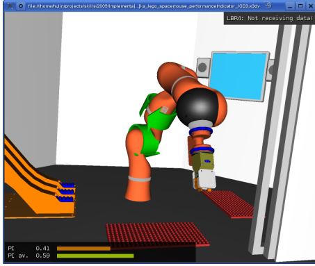
Figure 9: Visualization window of the Training-Center Setup, showing the performance indicator in the bottom-left corner, and rotating green arrows that indicate the direction of movement out of singular robot configurations.
