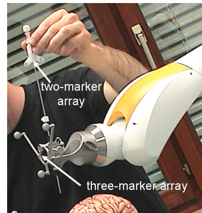
Fig. 2. Experimental set-up for the navigated biopsy with the medical robot KineMedic and the BrainLAB VectorVision navigation system.
