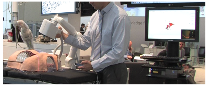
Fig. 4. The VR-Map is mounted to one of the medical robots and guided by hand to scan the patient dummy.
