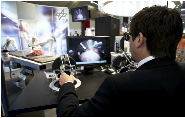
Fig. 2. The teleoperator station for the surgeon with two haptic master devices and a stereo display.
