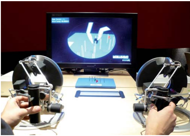
Fig. 10. Training a pegboard with haptic feedback and stereo imaging with polarized light.
