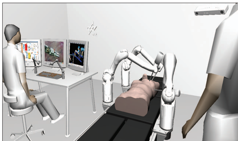
Figure 1. Schematic illustration of the DLR teleoperated surgery system for MIS. In the front, an assistant surgeon (e.g., for the application and change of instruments) is with the patient. In the background, the surgeon at a master console is directing the instruments.
