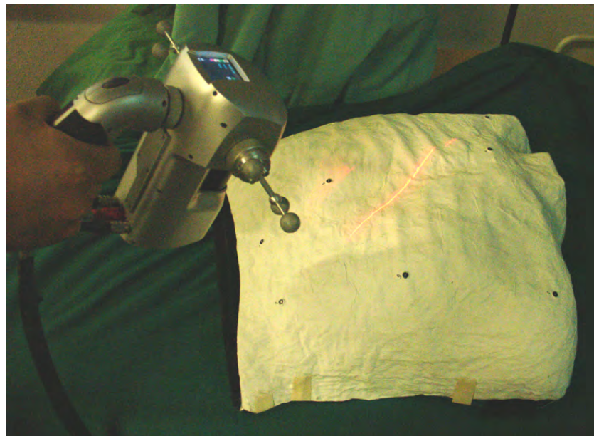
Figure 6.20.: Intraoperative scan of the patient for markerless registration with the hand-held 3D-Modeller.
