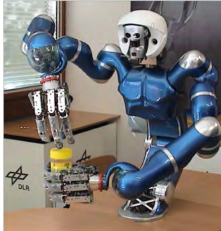
Figure 5.6.: The inverse kinematics is used to calculate the paths in tasks such as serving tea.
