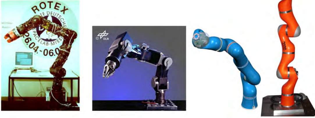
Figure 3.10.: The DLR Light-Weight Robot (LWR) generations (from left): LWR I (1991), LWR II (1998), LWR III (2002) and the commercialized version of the LWR III (2006).
