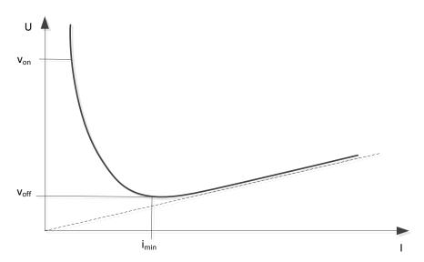
For the ignition of a light arc, a high voltage is needed. This "dielectric strength" is typically 25kV per cm of air gap. Once the arc has ignited, a plasma basically creates a short circuit between the two contacts. The resistance decays with increasing current and the characteristic curve has a hyperbolic regime which prescribes the minimum power needed to sustain the arc (U\*I = const). For higher currents the characteristic curve resembles the one of an Ohmic resistor.
