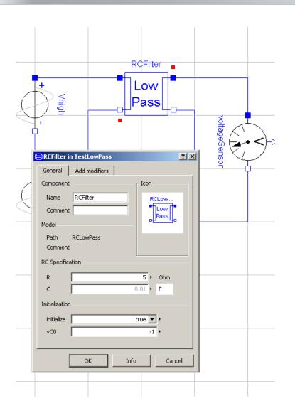
Within an electric circuit, the modeler can select the components he wants to initialize.
