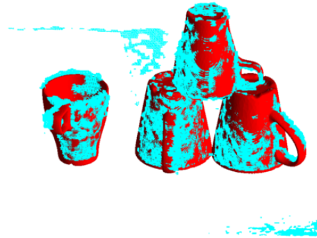
Figure 2: Point clouds (cyan) from a Kinect camera together with best matching models (red).
