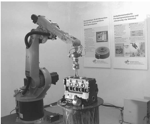
Figure 1: Overview of our assembly cell with rotating engine block and non-circular pistons
